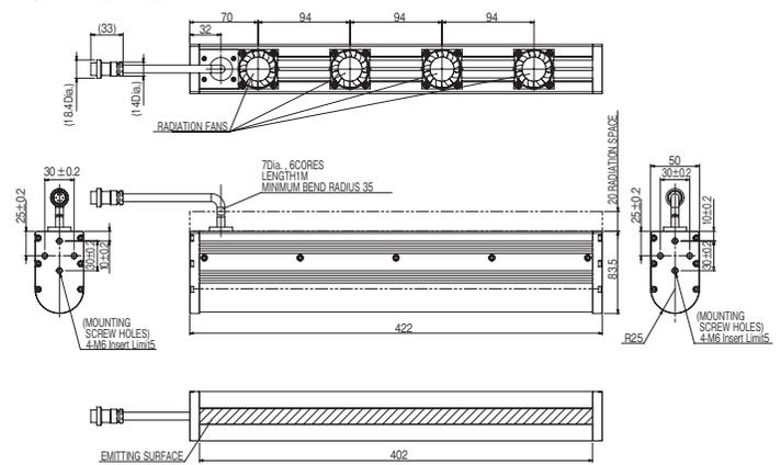
Tightening torque: 4.30N · m
