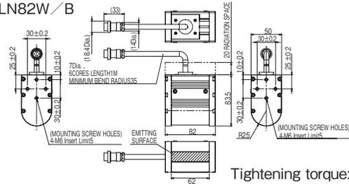
Tightening torque: 4.30N · m
